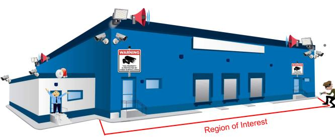
A CCTV camera is installed at the entrance / exit of the warehouse building, drawing a digital boundary or Region of Interest (RoI) in the camera view to cover the entrance / exit.
